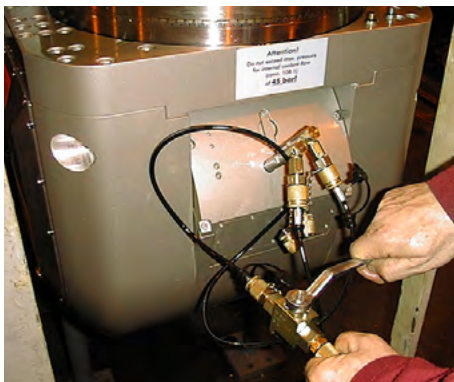
Bleeding set with closed blocking tap, attached to the ports of the clamp and release line on the swivel housing of the milling head.
